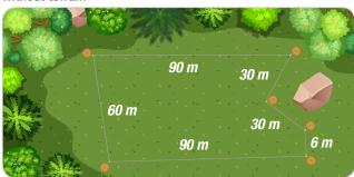
This pasture measures 306 m and includes a gate and must also bypass a large boulder. Therefore 6 stable corner posts are needed. For the partly long distances between the posts, line posts should be placed at intervals of 3 m, which keep 3 levels of wide tape at the same height (further post distances p. 7). For a fence length of 300 m you will need 100 line posts, but this does not include the length of the gate (6 m below the boulder here).
